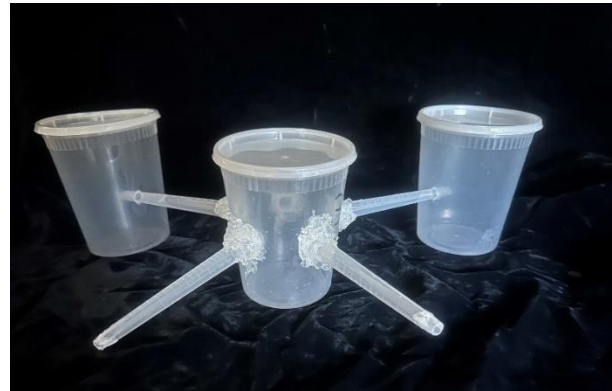
Fig. 3. Olfactometer used to determine adult sweetpotato weevil attraction and repulsion to volatiles emitted by sweetpotato with or without ‘Ko-002’.
