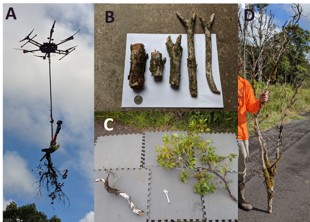
Figure 7. Aerial branch sampling. (A) Kūkūau branch sampler in the air following a successful cut; (B) Samples from a single branch, U.S. Quarter dollar (25 cents coin) for scale; (C) Two different collected branches, branch on the right contains healthy green leaves from a tree exhibiting partial C. lukuohia canopy symptoms; (D) >2 m tall branch collected by the Kūkūau branch sampler.
