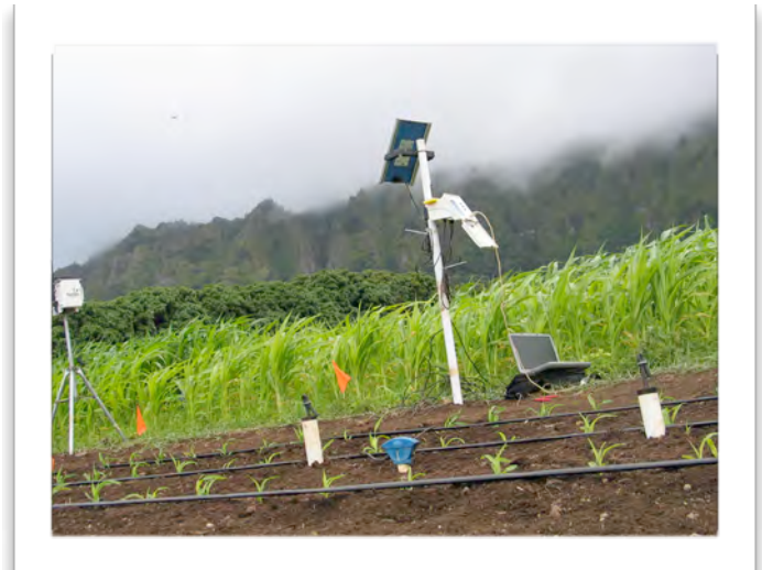
Figure 2. A plot of the compost treatment with drip irrigation system, two soil solution collection cups, a soil water content monitoring probe and its logger, and a weather station.
