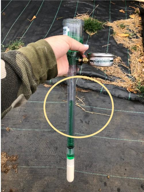
If air is permitted to flow down the plastic tube, false readings can occur (**Photo 6**). The final task is to fill the tensiometer reservoir with the fluid for the device along with removing air that may have accumulated in the reservoir. (Victoria State Government, 2009).
