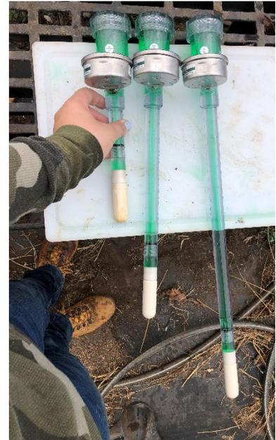
**Photo 1.** Examples of tensiometers at various lengths.
