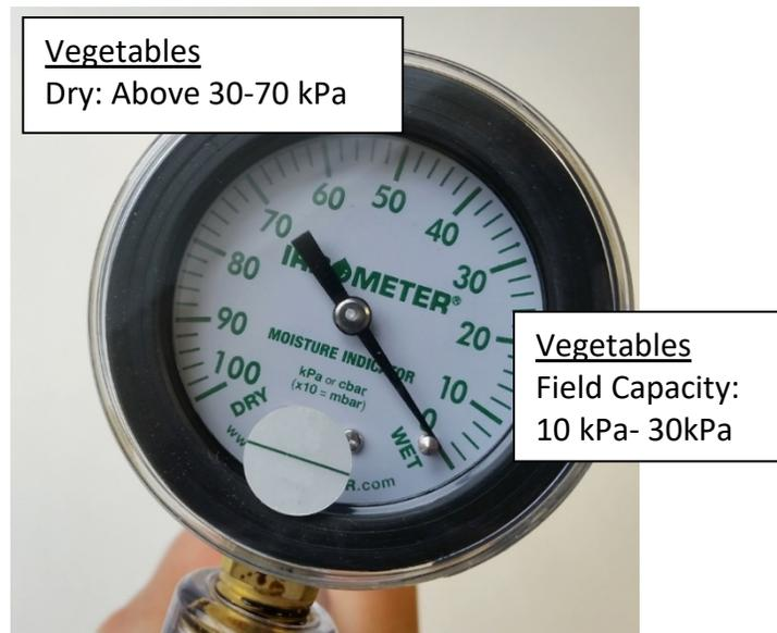
**Photo 4.** Commercially available tensiometers convert kPa values into positive values for ease of use. Photo credit: boutiquepro.ghlinc.com
