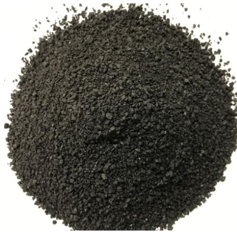
**Figure (3):** Biochar produced in Hilo from Macadamia nutshell.
