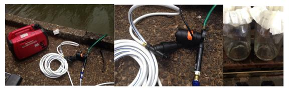
3<sup>rd</sup> filter as a coffee filter to mimic sand filter. Utilize chlorine and ORP meters
