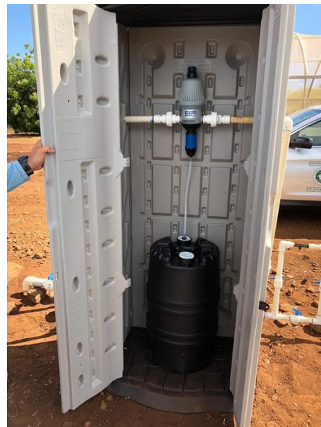
Pictured Above: The injector and system set-up used in demonstrations. Please contact a professional engineer to determine the proper equipment for your farm
