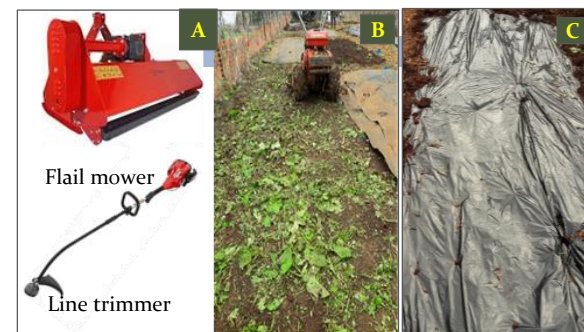
Fig. 4. A) Flail mower and line trimmer; B) hand-held rototiller incorporating macerated tissues into soil; C) cover the soil with black plastic mulch.
