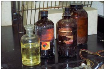
Moisture, high humidity, and long storage can damage boxes and bags, corrode cans and drums, and make pesticide labels unreadable. Photo University of Kentucky, Occupational Health and Safety
