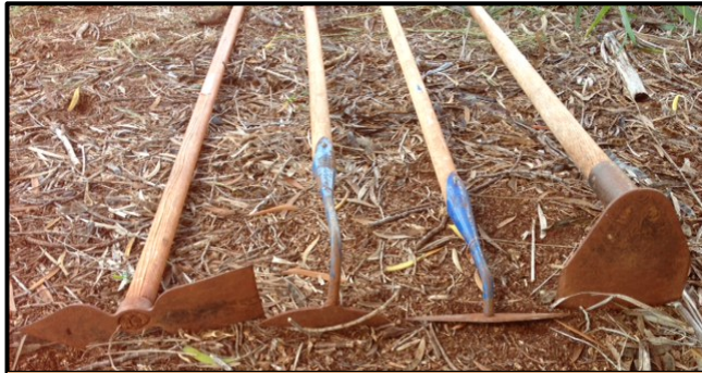
SHW chopper/row maker, DeWit half moon/swan neck hoe DeWit diamond scuffle hoe, and Rogue chopping hoe
