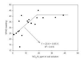
Figure 2. Relationship between SPAD readings and soil-solution NO<sub>3</sub>-N at 30-cm depth.
