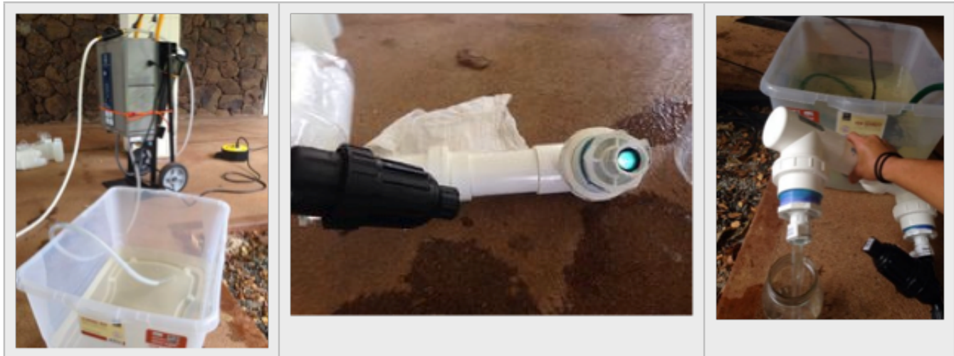
Aqueous ozone and UV system used.
