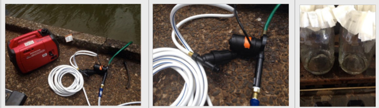
Irrigation water pumped into water containers with 2 inline filters. Used a 3rd coffee filter to mimic sand filter.
