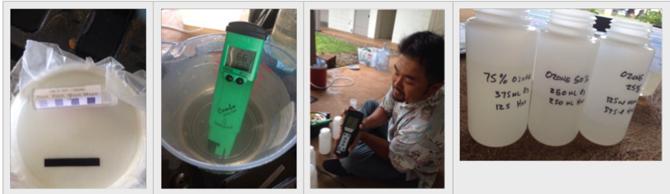
Calculated dosage and utilized chlorine strips, ORP and ATP meters to verify (and calibrate). Samples were submitted to the lab on the same day.
