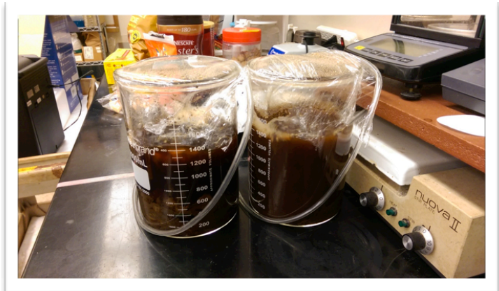
Fig 2. Brewing vermicompost tea overnight with air pumps (2.5W).
