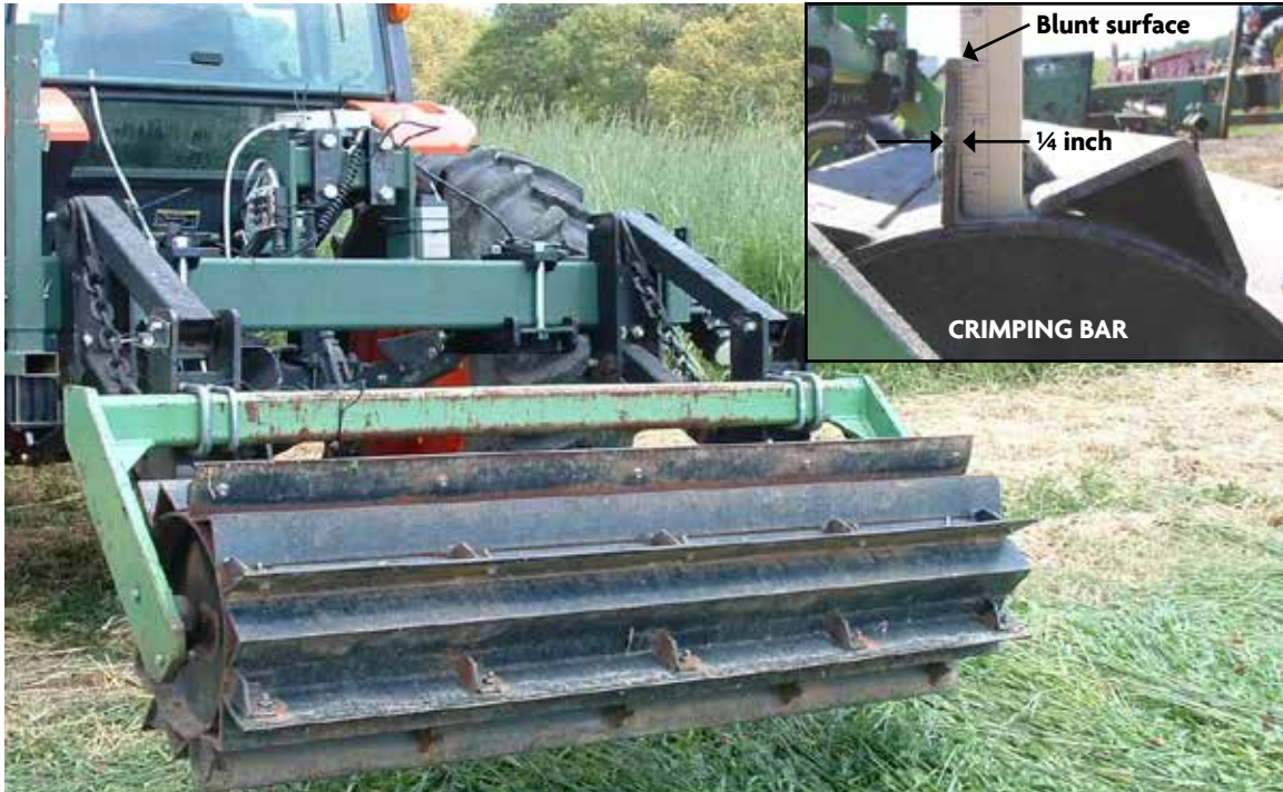
FIGURE 9.2. Brazilian-type roller/crimper with a detailed look at the height of the crimping bar.
