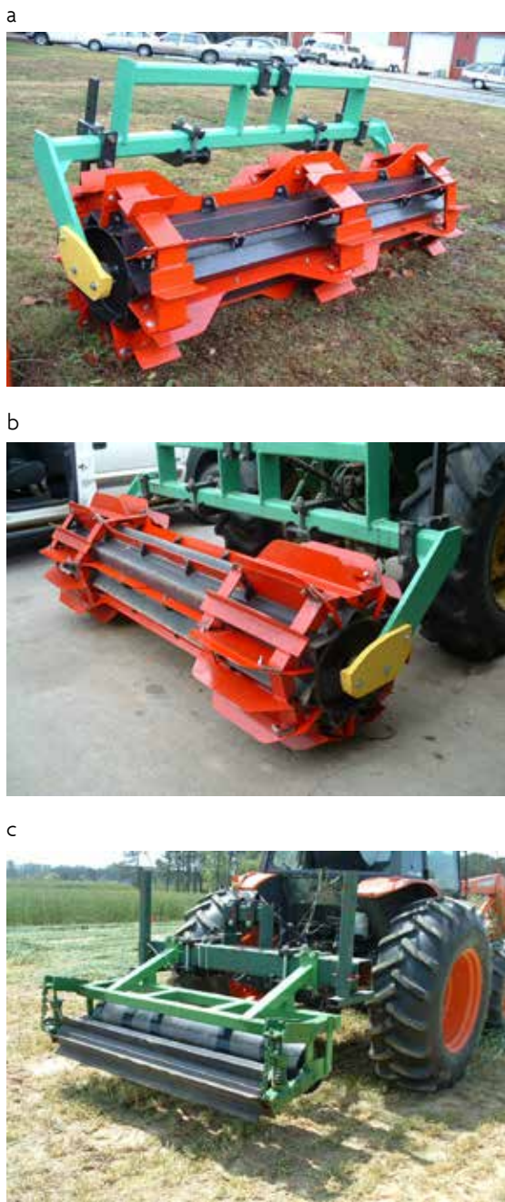
FIGURE 9.4. Roller/crimper for raised beds: (a) two rows and three furrows, and (b) one row and two furrows. A two-stage roller/crimper for smaller tractors (c).
