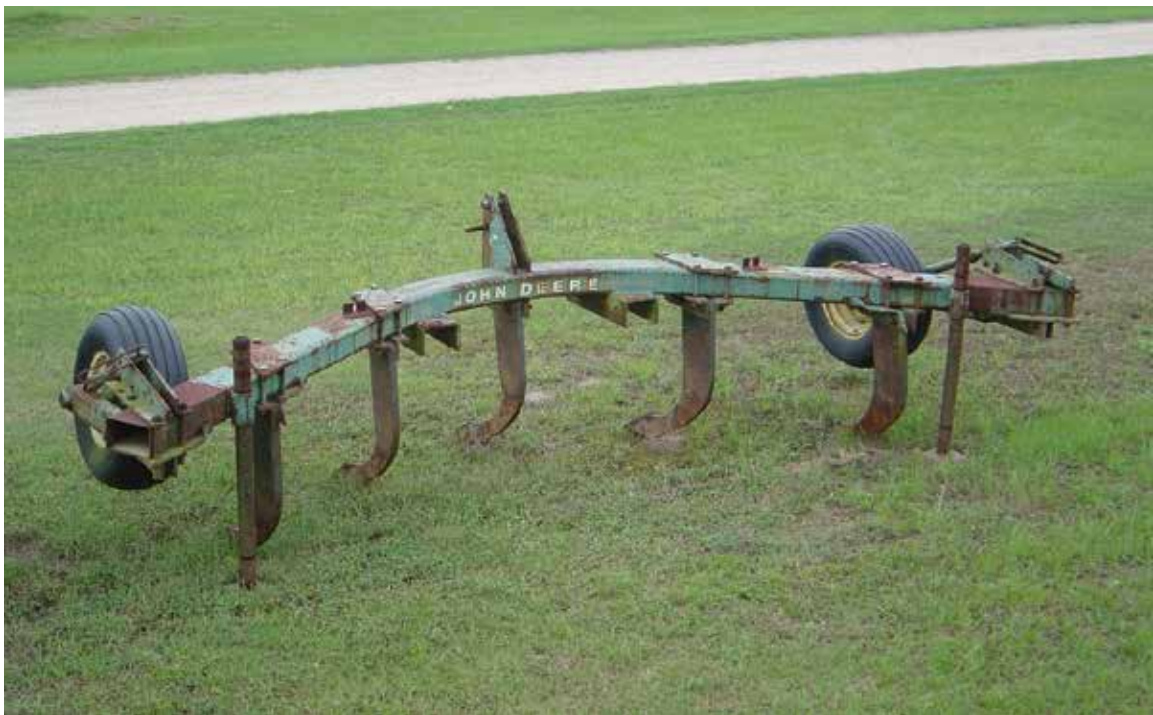
FIGURE 6.1. V-frame subsoiler used for soil disruption over the entire field. The shank spacing and depth are adjustable.
