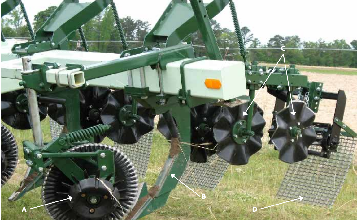
FIGURE 9.8. Wide-strip subsoiler. Picture shows (a) a narrow fluted coulters with attached row cleaners on the front of the shank, (b) splitter points attached to the shank, (c) additional coulters (ripper type) and (d) a drag chain sheet.
