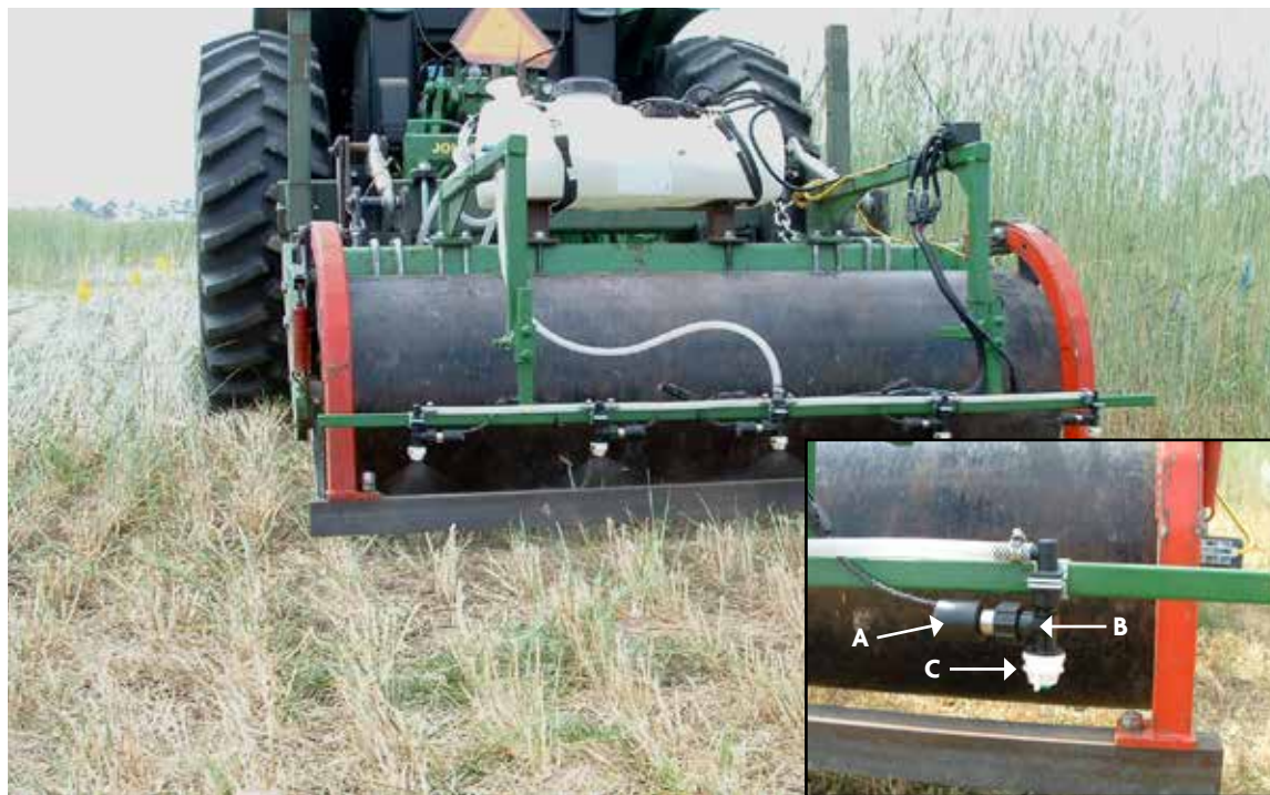
FIGURE 9.6. Back view of the smooth roller with crimping bar and the attached high-speed solenoid valve; (a) solenoid valve, (b) nozzle body and (c) nozzle.
