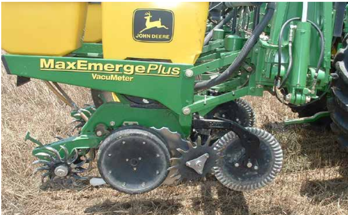
FIGURE 99. John Deere no-till planter for planting cotton seeds into rye residue using Dawn row cleaners.
