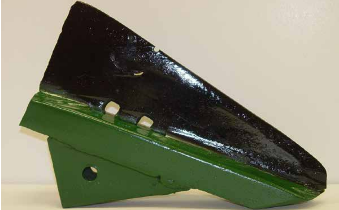
FIGURE 9.12. A splitter point is a black, sharp-edged plastic addition that looks like a shark fin and is attached directly to the tip of the shank point (see Figure 9.10).
