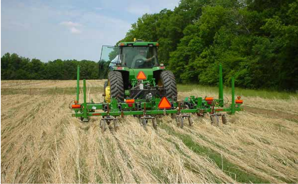
FIGURE 6.2. In-row subsoiling with heavy cover crop residue. Very little residue is buried or disrupted while in-row subsoiling.
