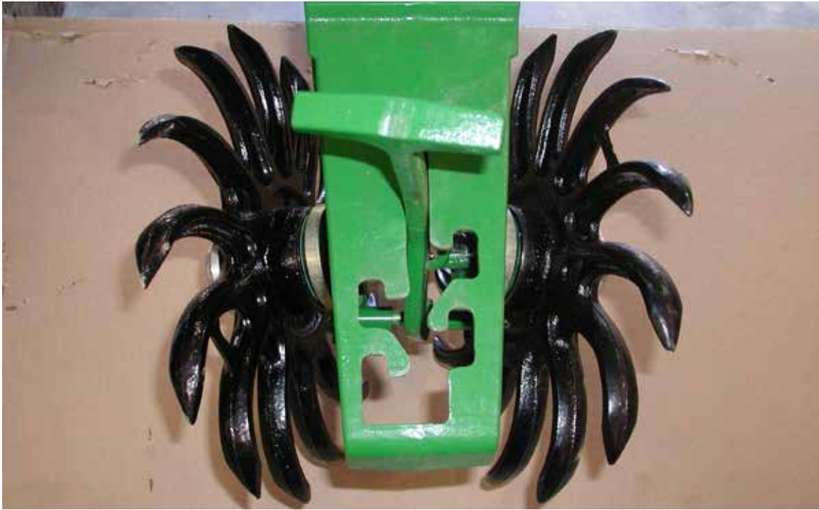
FIGURE 9.14. Top view of spoked closing wheels on a John Deere no-till planter.
