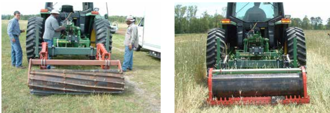
FIGURE 9.3. Rolling/crimping equipment: (left) spiral bar roller/crimper and (right) smooth roller with crimping bar.
