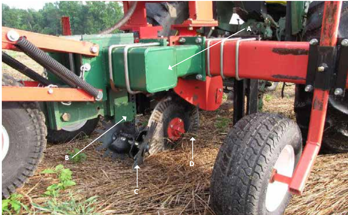
FIGURE 9.17. Close-up of the RJ transplanter showing (a) the subframe for the subsoiler (subsoiler removed) with (b) an attached custom-made bracket for proper positioning of (c) the row cleaners behind (d) the fluted couler.
