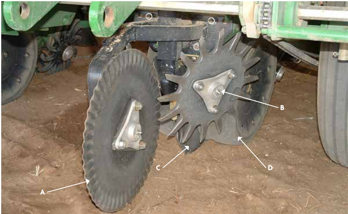
FIGURE 9.13. (a) Narrow fluted coultter with (b) the attached Dawn row cleaners for a John Deere planter. (c) Double disk openers and (d) gage wheels are also shown.
