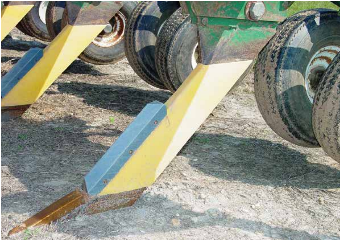
FIGURE 9.11. Plastic shield that fits over the shank to prevent soil from sticking to the shank, minimizing “blowout.”
