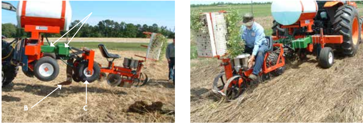
FIGURE 9.16. Side view of the modified RJ transplanter showing (a) the subframe with (b) the subsoiler shank and (c) two driving wheels to power the planting unit (left). Planting tomato seedlings into previously rolled/crimped rye using a modified RJ no-till transplanter from RJ Equipment Company (right).
