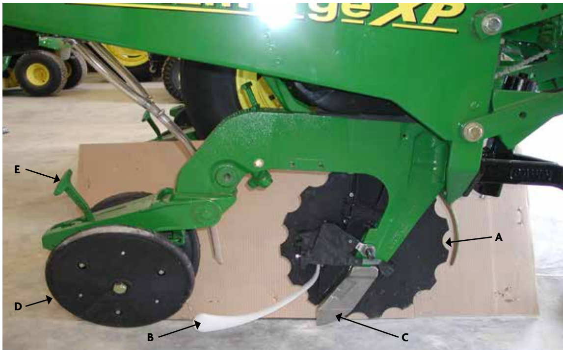
FIGURE 9.15. This John Deere no-till planting unit shows (a) a disk opener with a planting tube knife, (b) seed firmer, (c) V-slice insert and (d) press wheels with rubber tire assembly controlled by (e) a downward pressure adjusting lever.
