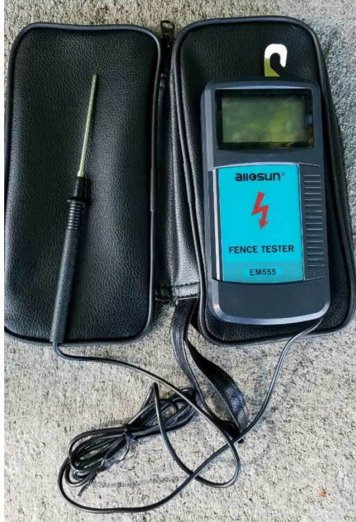
Figure 9. Example of a fence tester with a hook to hang it to the fence wires and a needle to connect it to ground.
