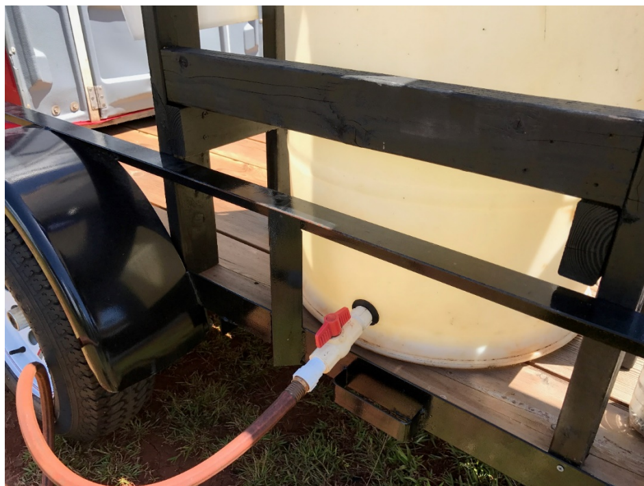
Dirty water catchment system and disposal hose
