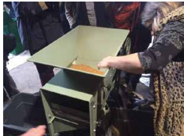
A seed intensive workshop demonstration using a winnowing machine to clean seed.
